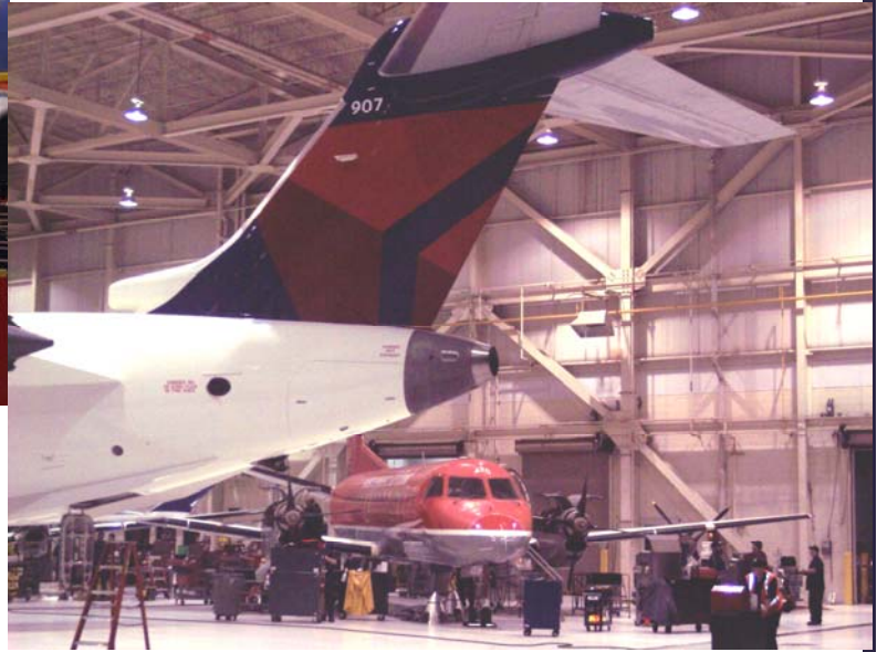
To the right a Mesaba Airlines SAAB 340 is being worked (backset) during a RON visit at the DTW Maintenance Hangar. Pictured in the front is the empennage of a CRJ-900 with the Delta Connection livery
